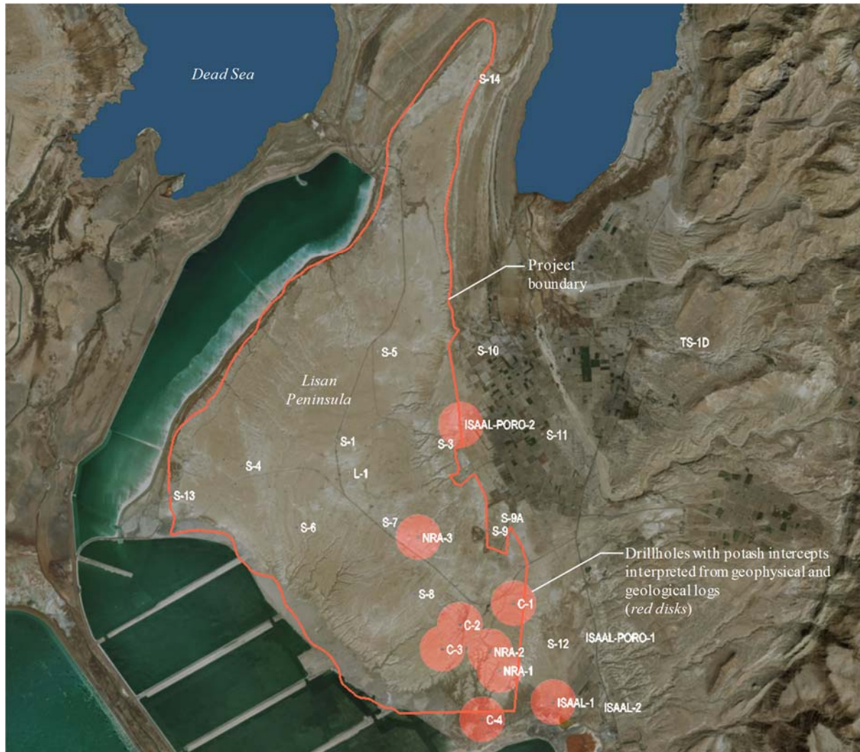
Figure 9-21. Drillholes with Potash Mineralization ( underground view to north )
