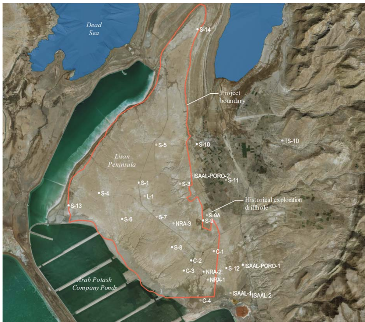
Figure 9-6. Historical Exploration Drillholes in Model (plan view)
