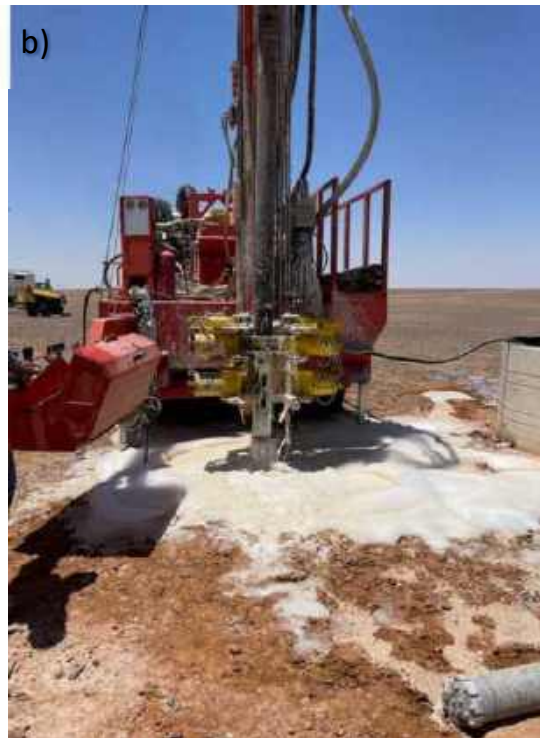
Figure 4: a) Phosphate Risha Study Area, b) Core Drilling at Study Area
