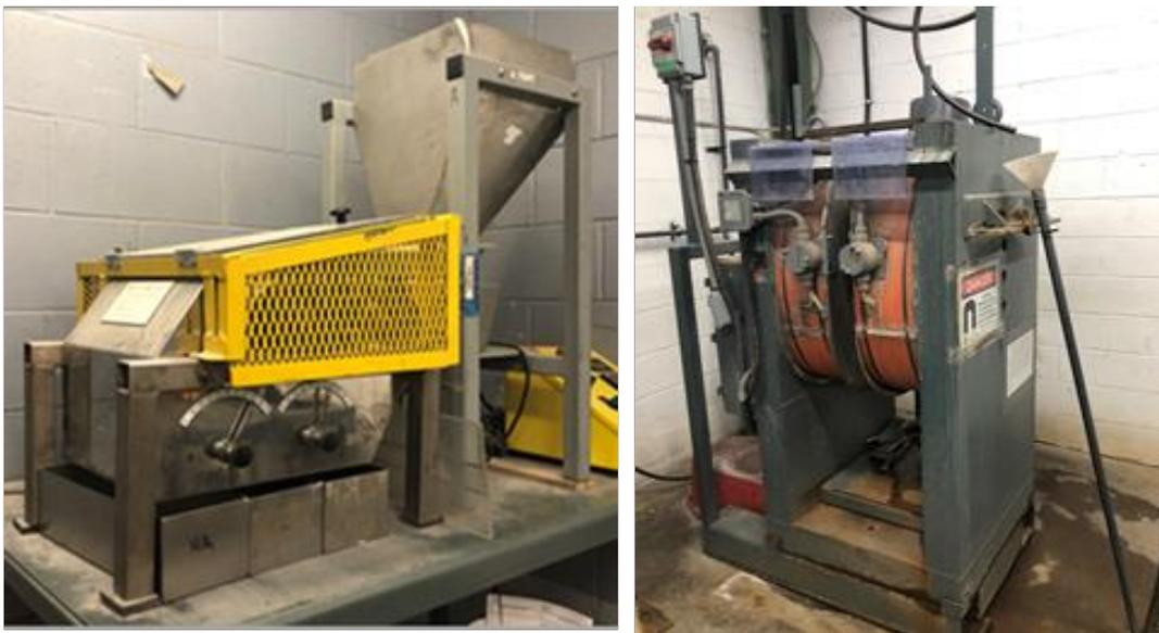
**Figure 5: Exhibition of Dry Magnetic Separator (left) and Eriez WHIMS Lab Unit (right)**
