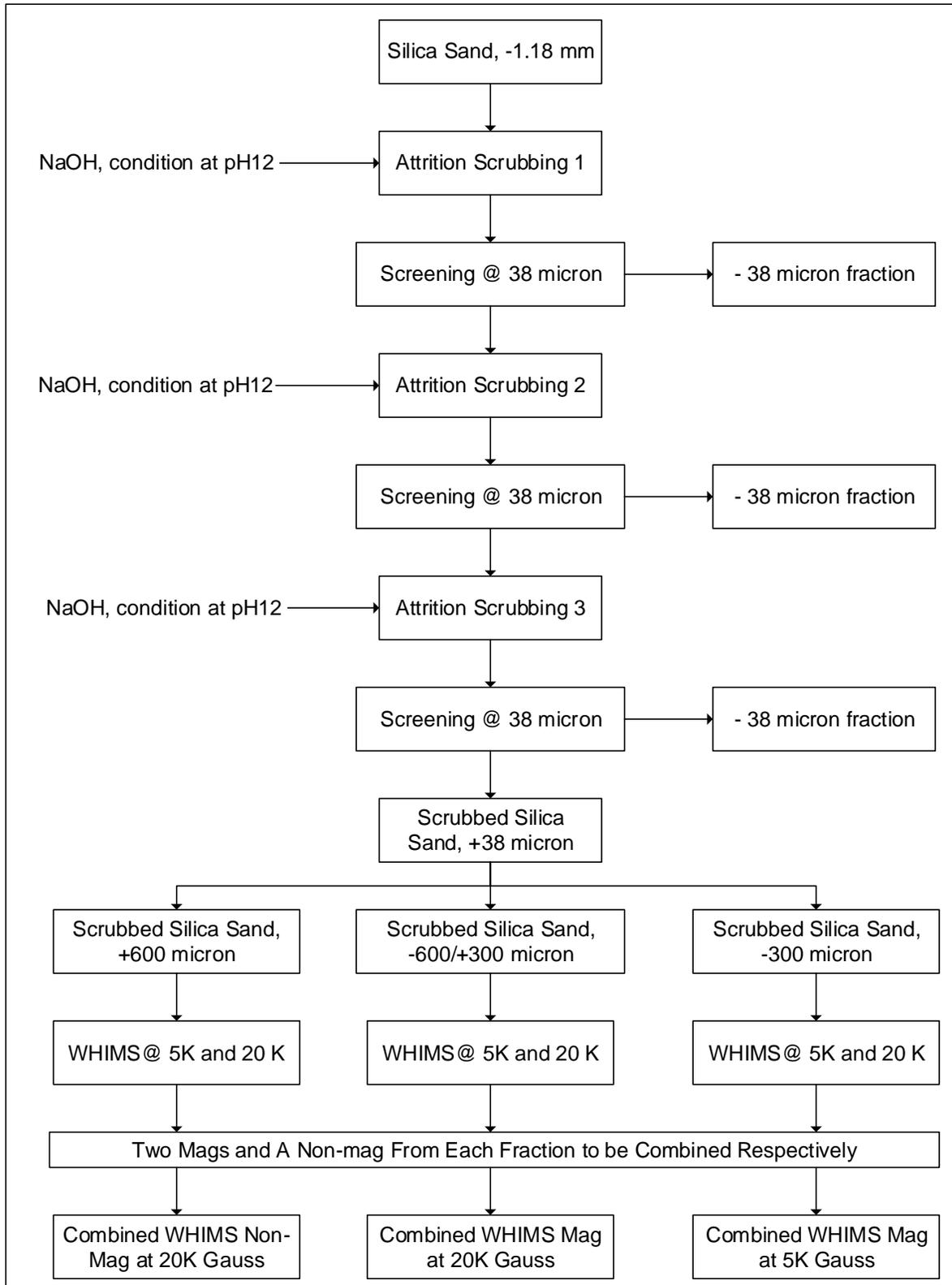
**Figure 6: Block Flow Diagram of Three-Stage Attrition Scrubbing and WHIMS Testing**
