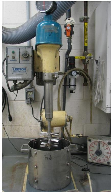
Figure 3: An Image of Multi-blade High Intensity Scrubbing Unit
