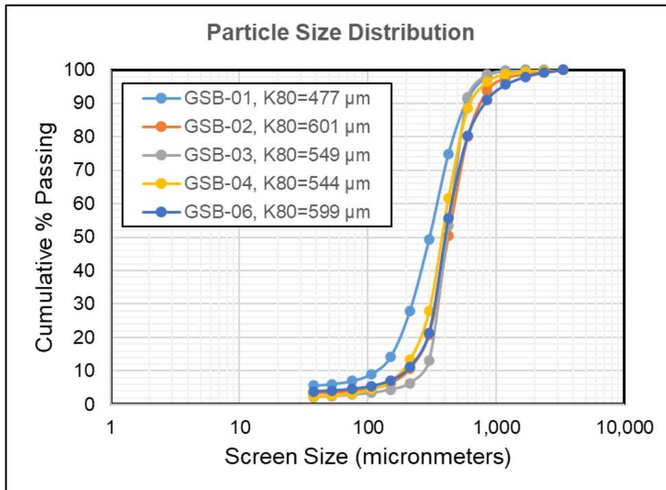
Figure 1: Particle Size Distribution of Five Silica Sand Samples
